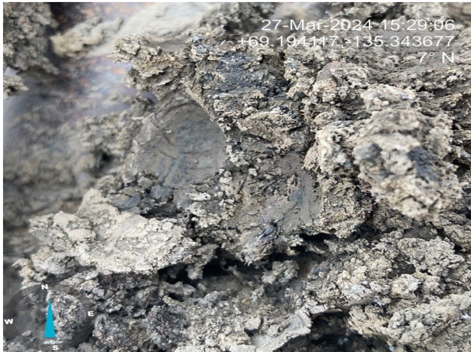
Photo 27 – Soil from BH24-31 at 1.5 mbgs with black stain and hydrocarbon odour (27 March 2024).
