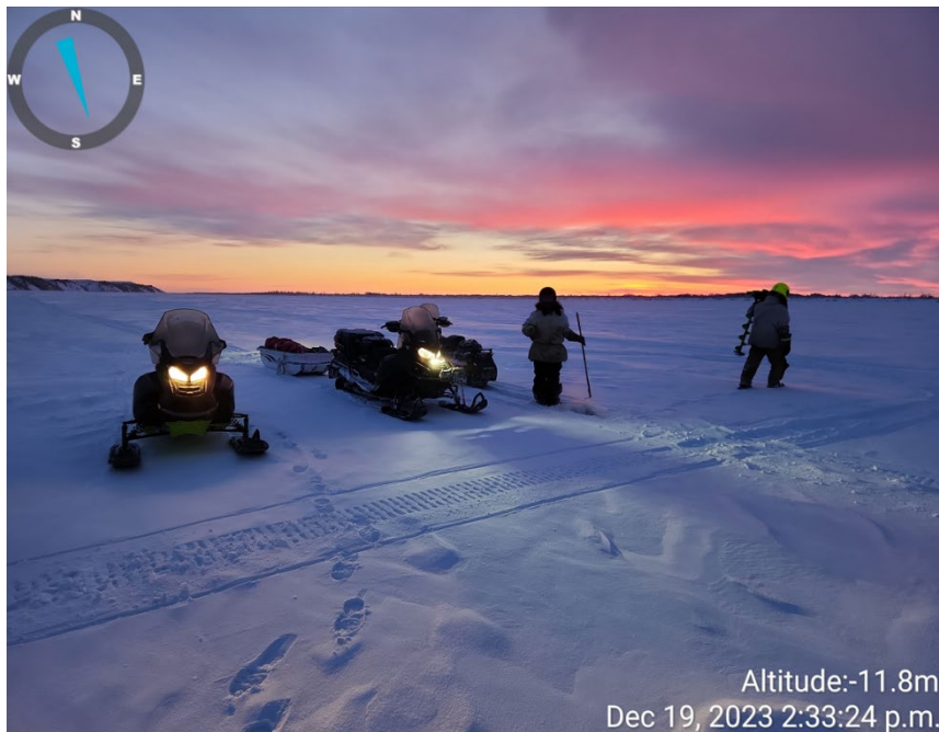
Photo 12 – Ice Road Pre-Construction - Crew completing ice thickness measurements by snowmobile (19 December 2023).
