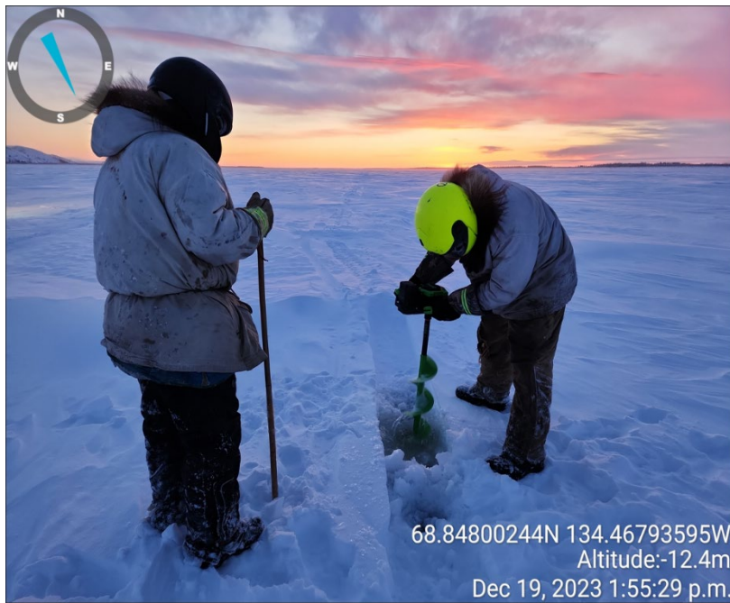
Photo 11 – Ice Road Pre-Construction - Ice thickness measurements along proposed route (19 December 2023).
