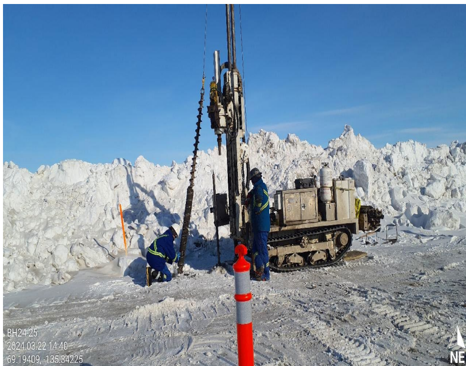
Photo 26 – Collecting soil sample from an auger at BH24-25 (22 March 2024).
