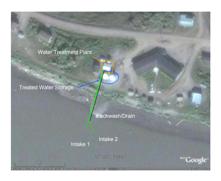
Figure 2. Water Supply Site Plan
