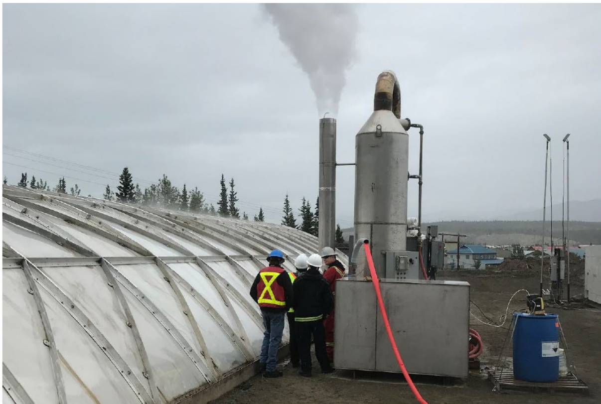
Photo A: Example quench tower in operation at an unrelated site.
