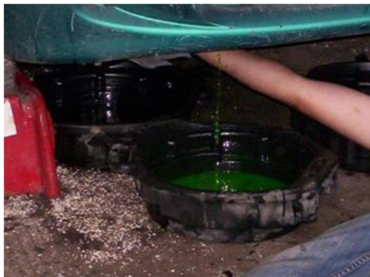
Figure 3: Using Pans to Catch Draining Fluids
