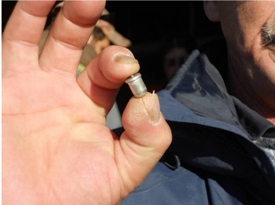
Figure 11: Mercury Pellet from Vehicle Convenience Light Stockpiling
