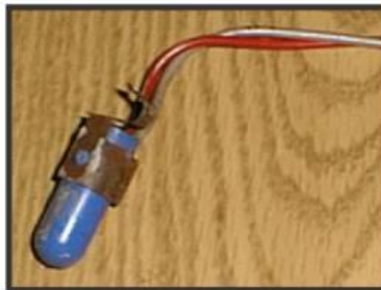
Figure 7: Washing Machine Mercury Switch (Source: Vermont Department of Environmental Conservation et al., 2002)
