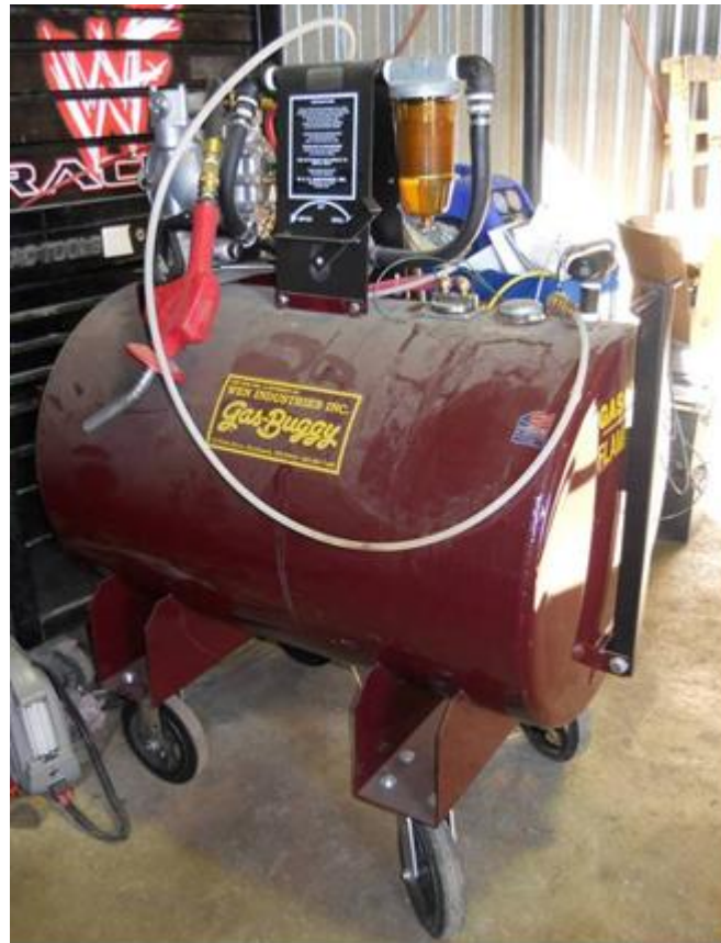
Figure 2: Example of Gasoline Collection System
