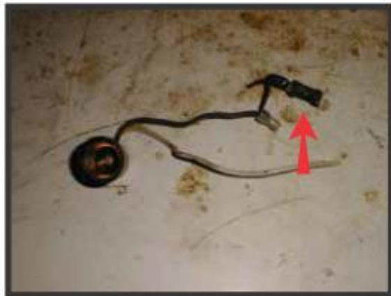
Figure 3.13: Chest Freezer Light with an Inline Mercury Switch (Glass Ampule)
