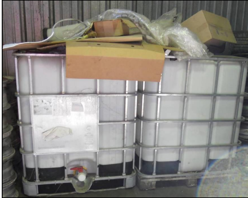
Figure 3.5: Example of Plastic Totes Used for Collection of Vehicle Fluids - Not Used for Gasoline
