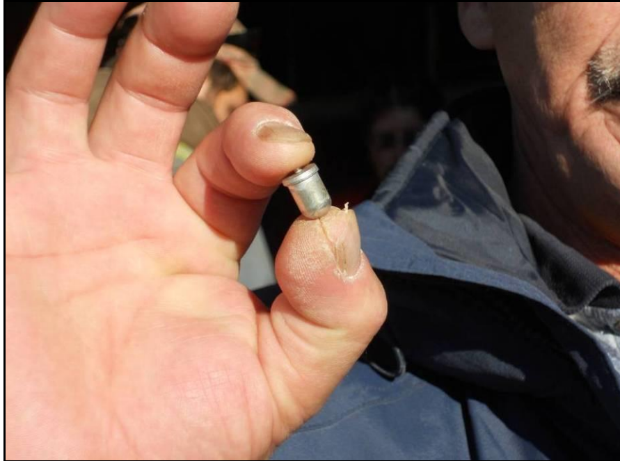
Figure 3.18: Mercury Pellet removed from Vehicle Convenience Light
