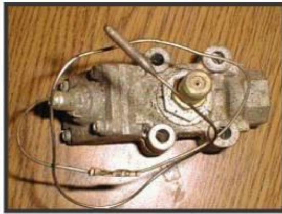
Figure 3.15. Gas Safety Valve Control, Gas Safety Valve Capillary Tube and Safety Valve Sensor Bulb from Gas Range
