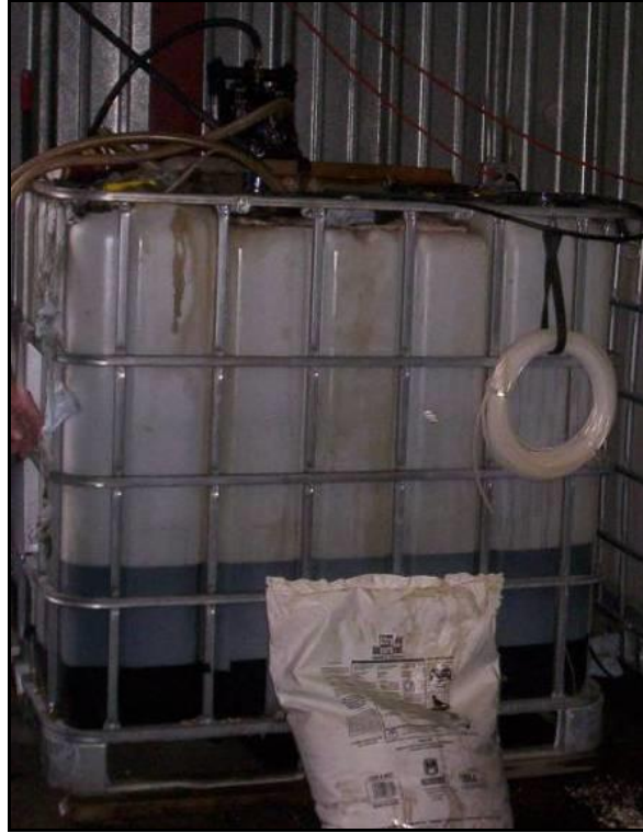
Figure 3.11: Example of Plastic Container Used for Storage of Waste Oils
