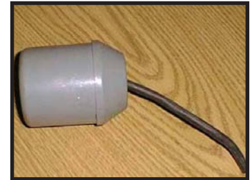
Sump pump float containing mercury.
