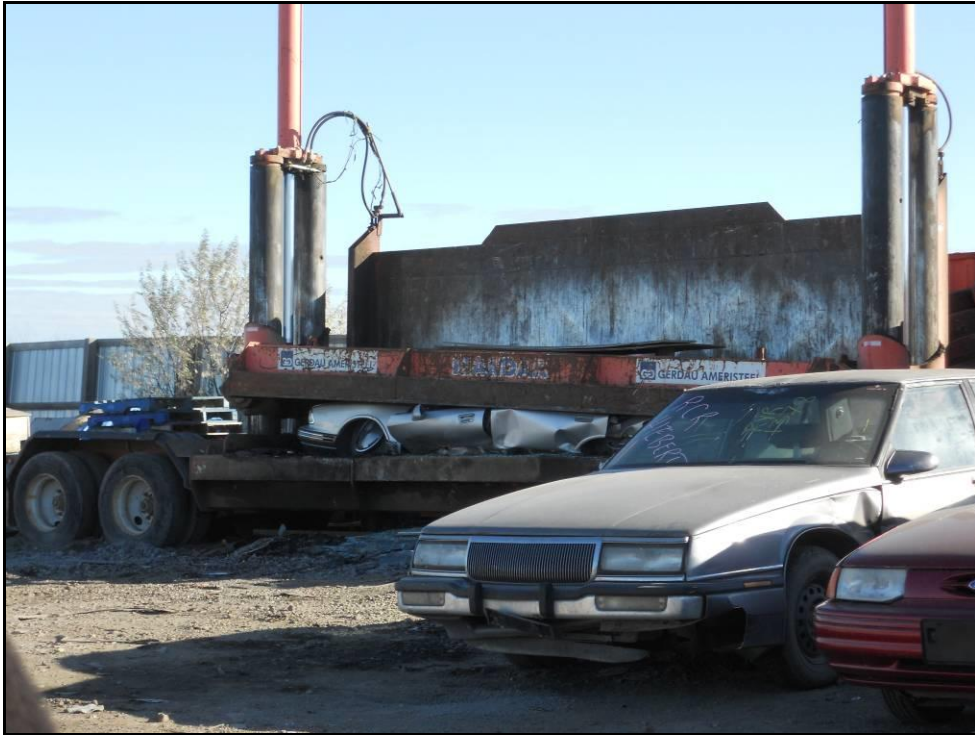
Figure 3.6: Vehicle Crusher in Operation
