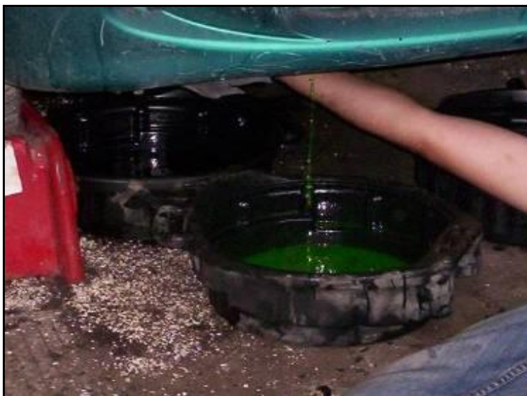
Figure 3.9: Using Drip Pans to Catch Draining Fluids
