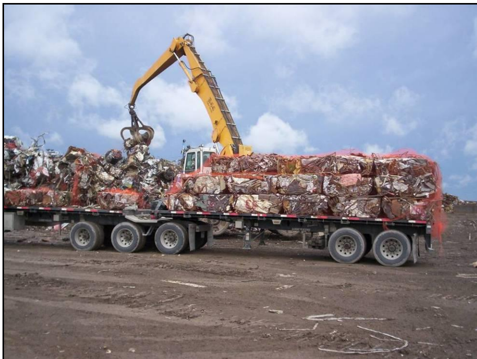
Figure 3.7: Example of "Logged" Metal
