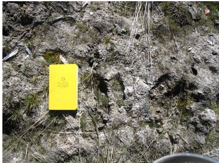
**Photograph 4:** Salt efflorescence observed in sump and off-lease spill area.
