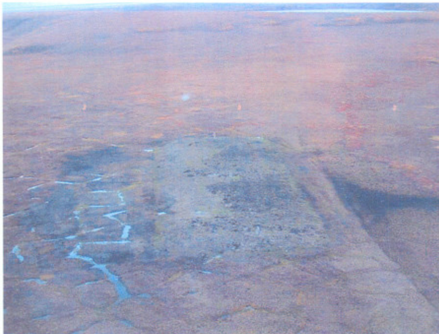
Plate 2. Aerial view of Umiak N16 sump (west end in foreground). Note thermistors down center axis of sump. (photo by Kavik-Axys)
