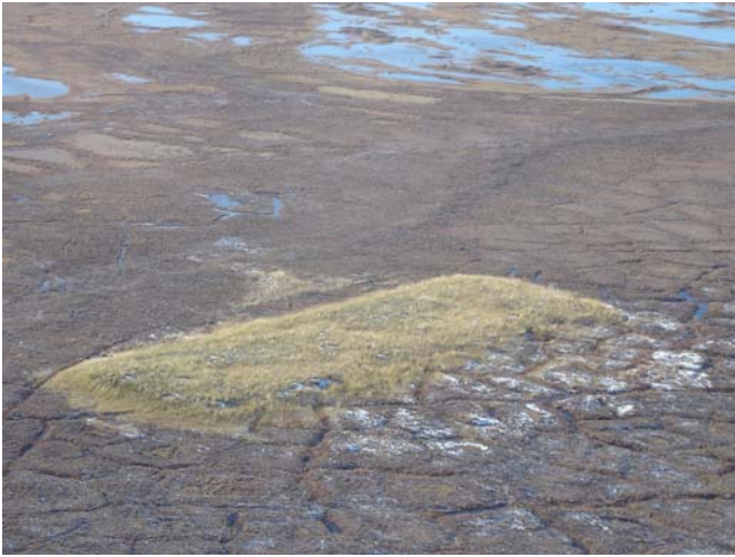
Figure 1 Aerial overview of drilling waste sump, from the northeast corner. Note the subsidence and polygons presence surrounding the sump.
