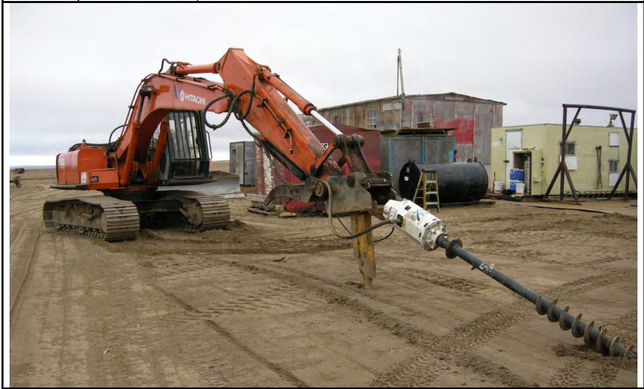
Photo 6: Soil sampling Auger equipment
