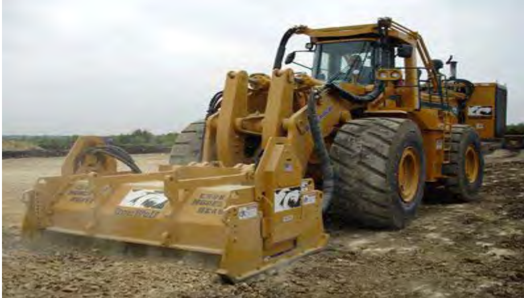
Photo 5-1: Proposed IronWolf™ Excavation Method
