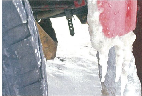
Figure 2 Water Truck dripping oil but was missing the belly tarp and a drip tray.
