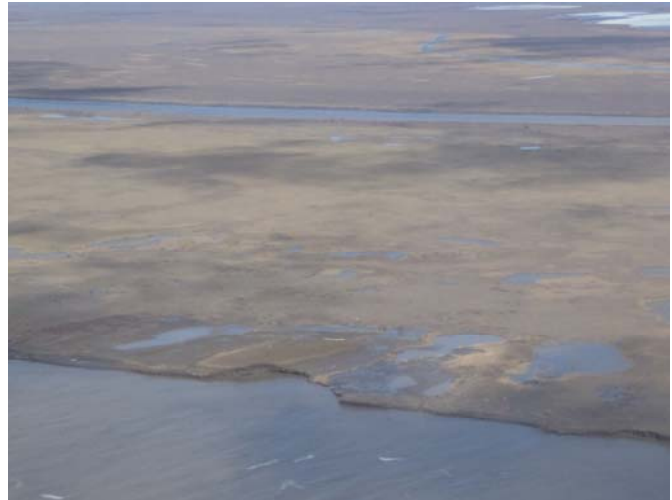
Figure 2 Unipkat I-22 sump was excavated then backfilled but now has erosion of the bank and former sump area, June 14, 2011 – DFO photo.
