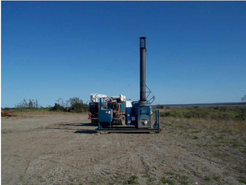
Photograph 15: Incinerator used to burn domestic waste produced by barge camp (August 17, 2014).
