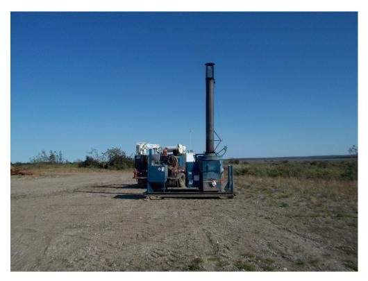
Photograph 15: Incinerator used to burn domestic waste produced by barge camp (August 17, 2014).
