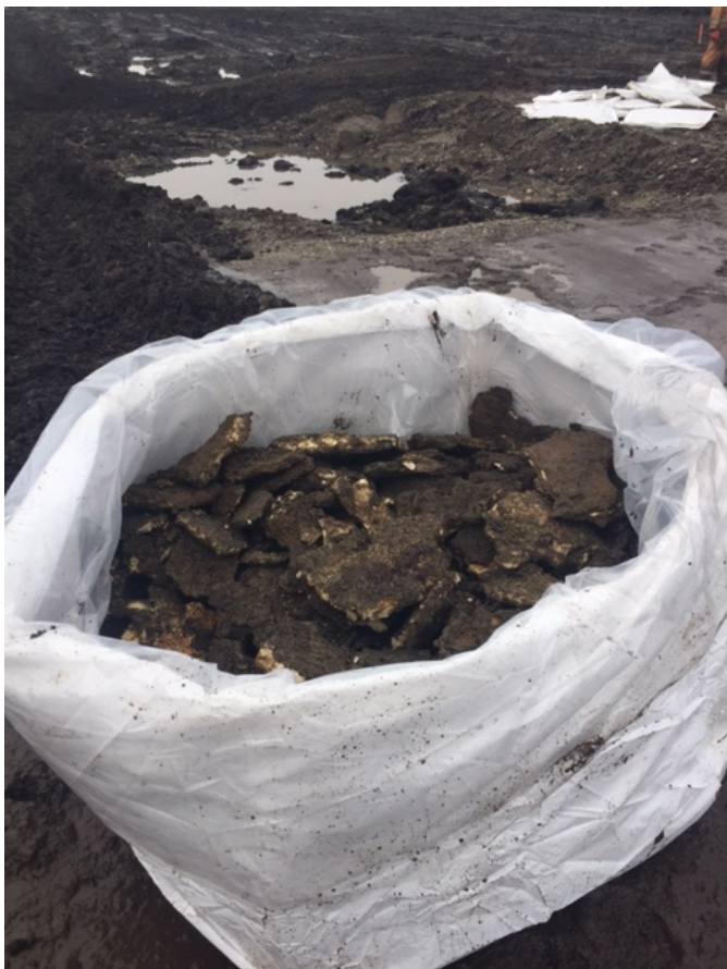
Photo 4 View of polyurethane foam in soil bag (September 6, 2018).
