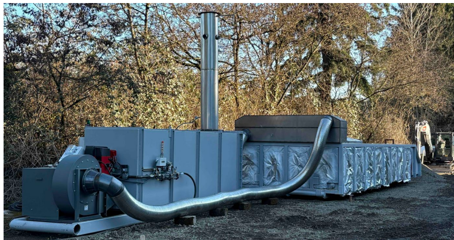
Photo 1: A single, operating TecZero thermal treatment unit connected to a thermal oxidizer.
