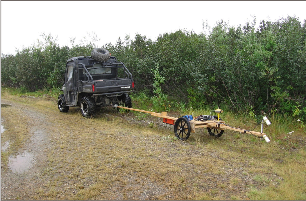
Photo 1: View of Geophysical Survey setup. All equipment was towed behind the side-by-side, mounted to a non-magnetic and non-conductive wooden cart.
