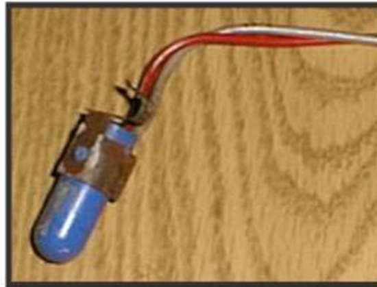
Figure 13: Washing Machine Mercury Switch (Source: Vermont Department of Environmental Conservation et al., 2002)
