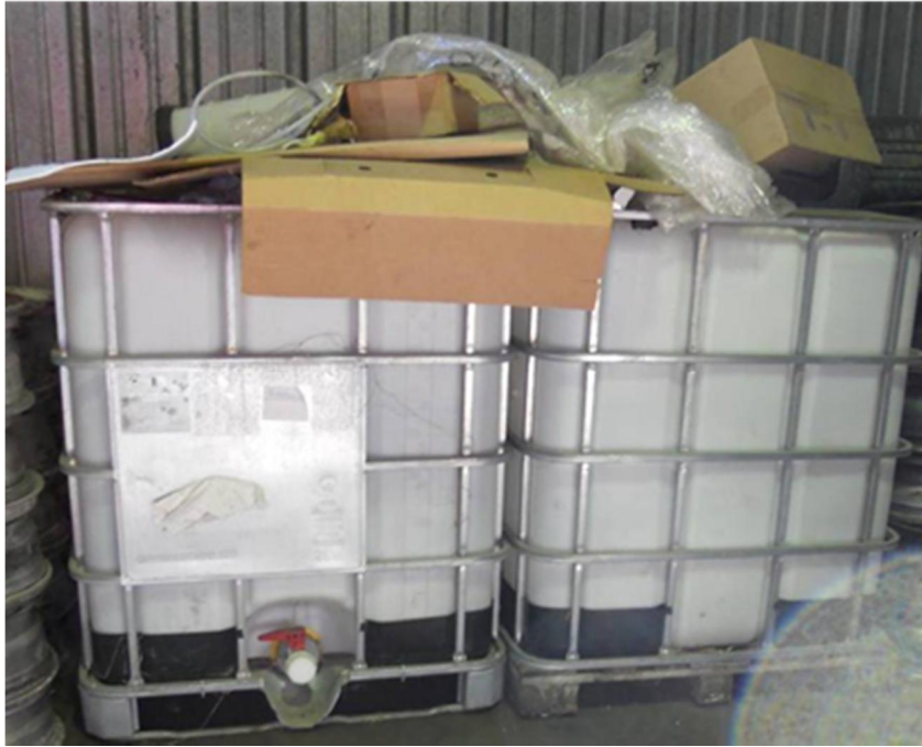
Figure 5: Example of Plastic Totes Used for Collection of Vehicle Fluids - Not Used for Gasoline
