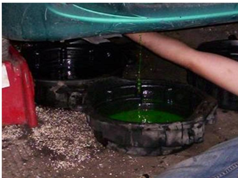
Figure 10: Using Pans to Catch Draining Fluids
