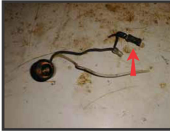
Figure 12: Chest Freezer Light with an Inline Mercury Switch (Glass Ampule) (Source: Vermont Department of Environmental Conservation et al., 2002)
