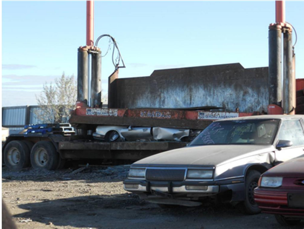
Figure 7: Vehicle Crusher in Operation
