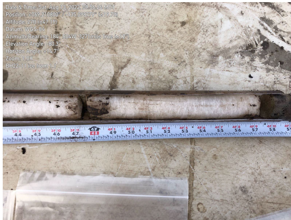
Photo 14 – Ice observed at BH22-11 (August 13, 2022).
