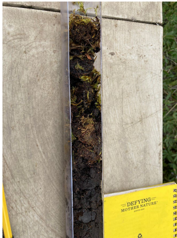
Photo 6 – View of the peat observed at BH22-42 (August 6, 2022).
