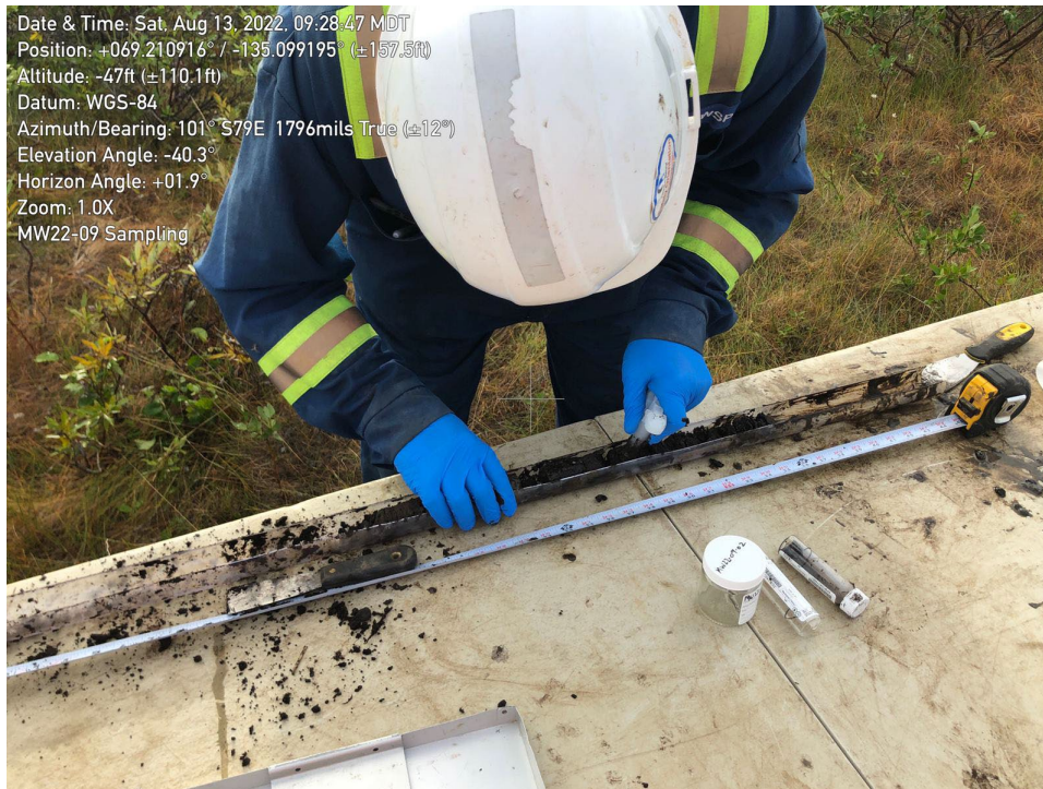
Photo 13 – Soil sampling at MW22-09 (August 13, 2022).
