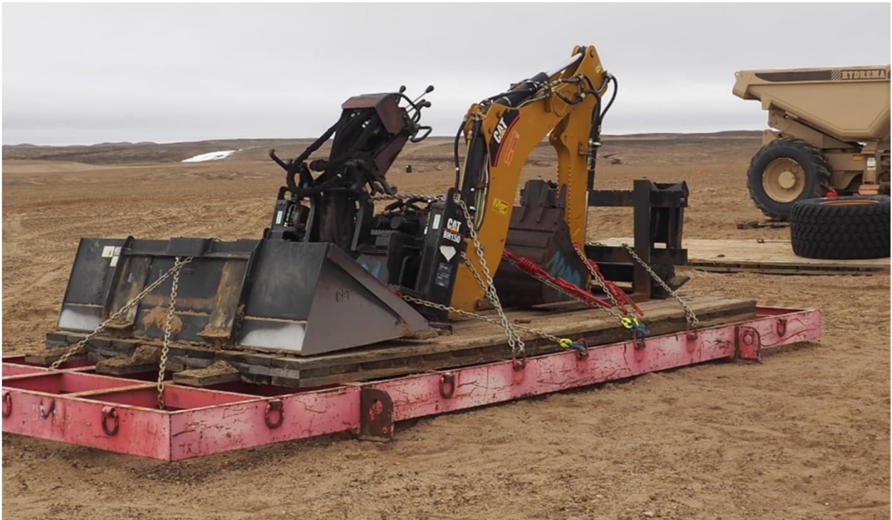
Photo 4 – Equipment load prepared on helicopter lift frame (18 July 2025).
