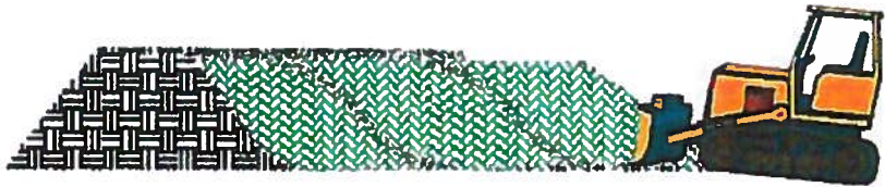
Compaction of consolidated waste
