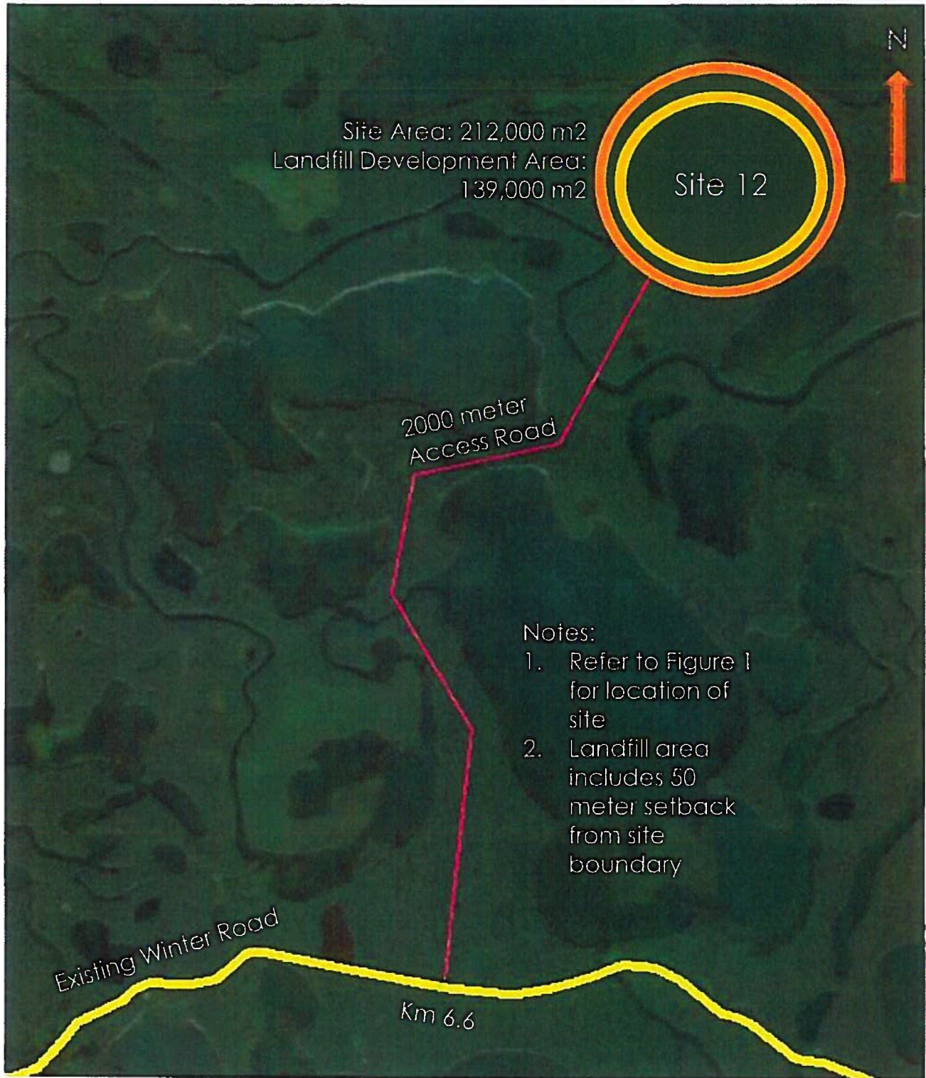
Hamlet of Aklavik, NWT Landfill Siting Study FIGURE 16. Site 12 - Envelope and Access Prepared by Jamie Davignon, B.A.Sc., EIT, 2016 06 21
