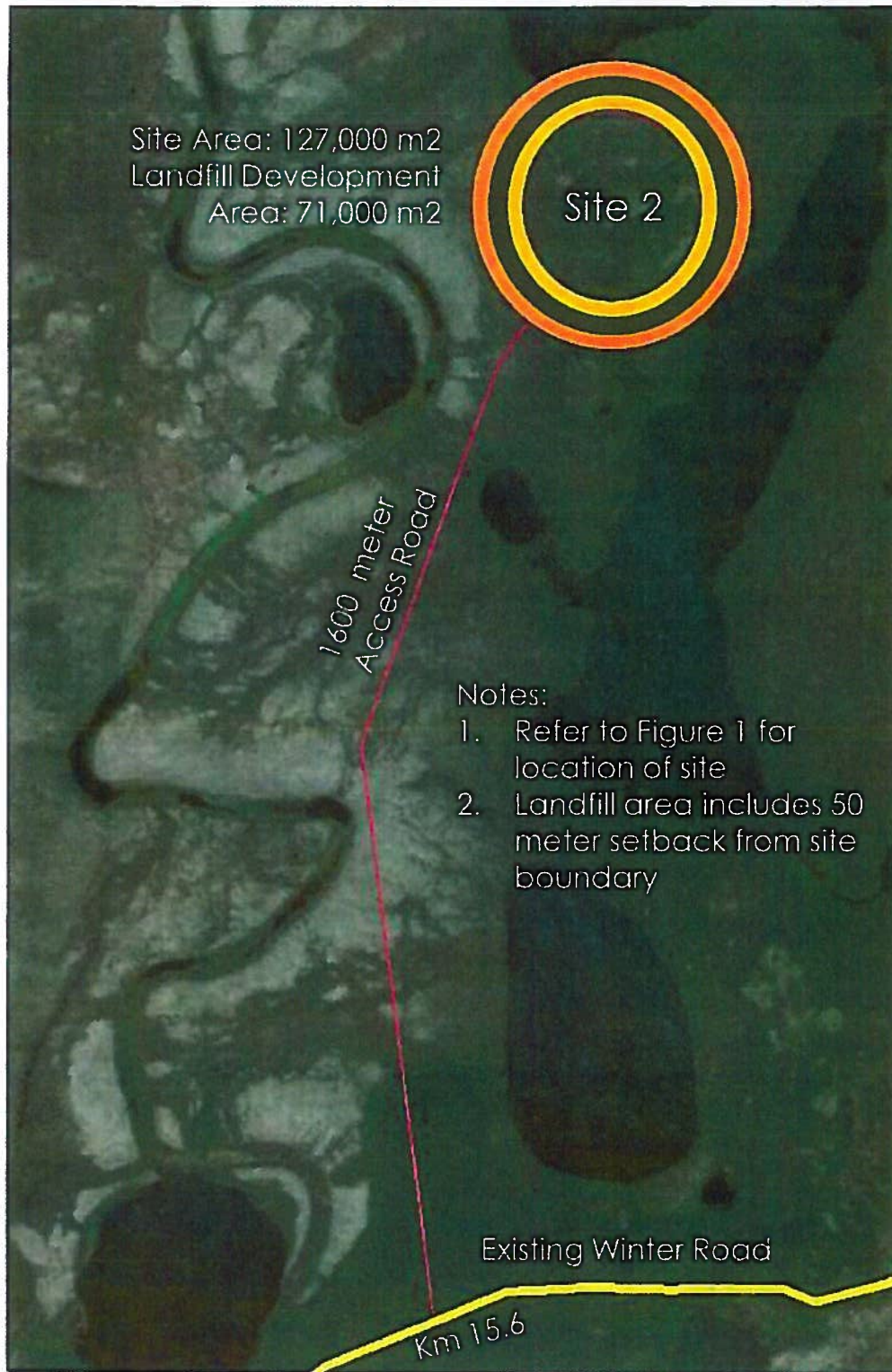
Hamlet of Aklavik, NWT Landfill Siting Study FIGURE 6. Site 2 - Envelope and Access Prepared by Jamie Davignon, B.A.Sc., EIT, 2016 06 21
