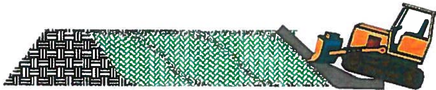
Compaction of intermediate cover
