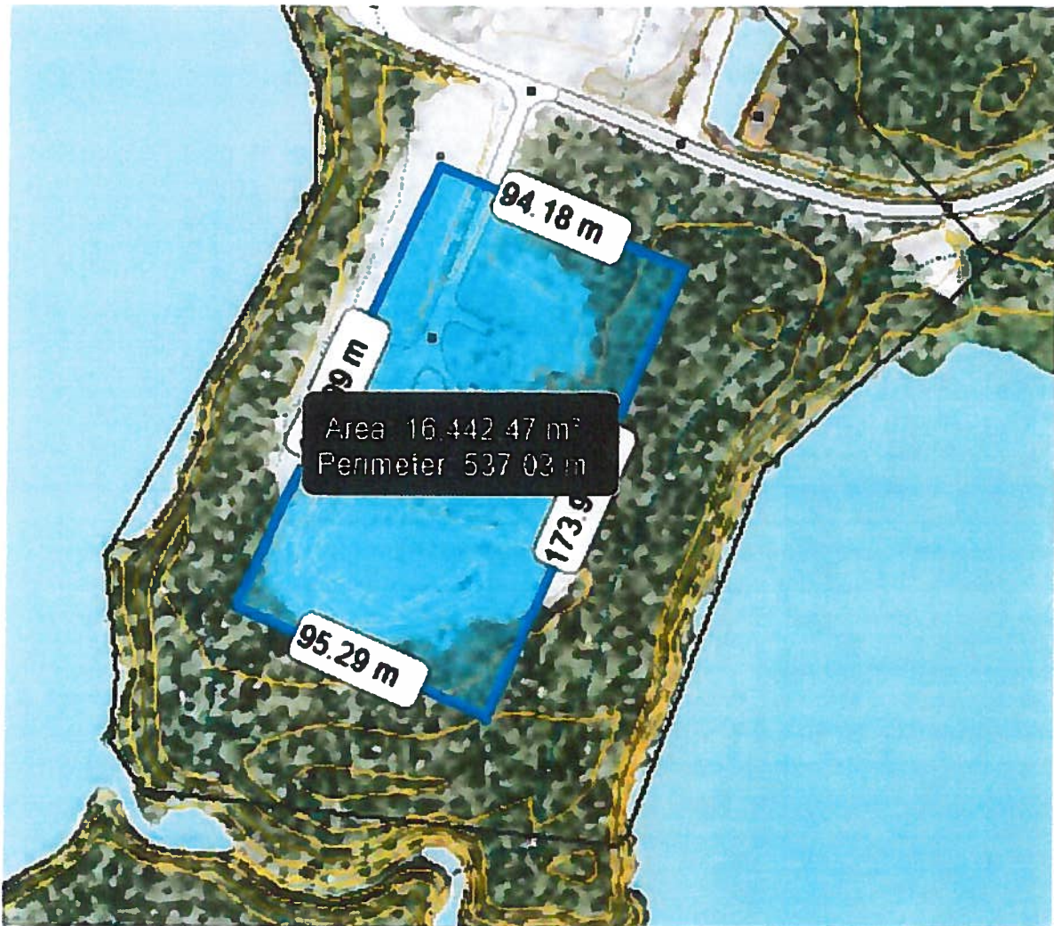
Figure 1: GNWT ATLAS image with a proposed landfill footprint of Est. 95 m x 175m
