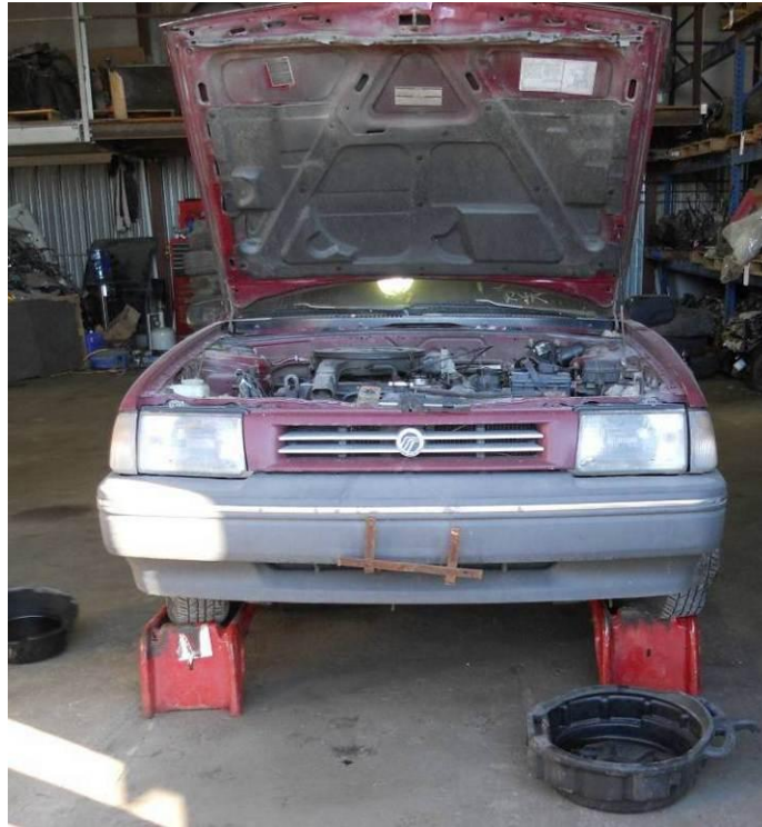
Figure 3: Vehicle Ready for Dismantling
