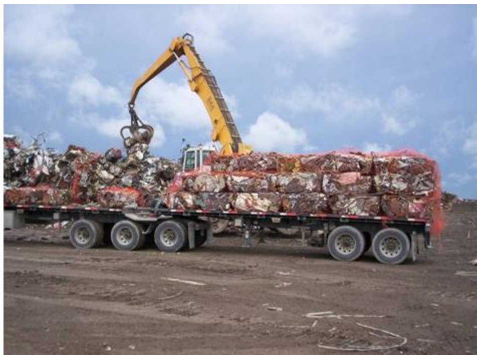
Figure 8: Example of "Logged" Metal
