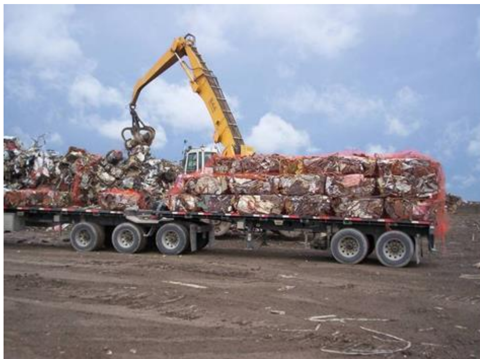
Figure 8: Example of "Logged" Metal
