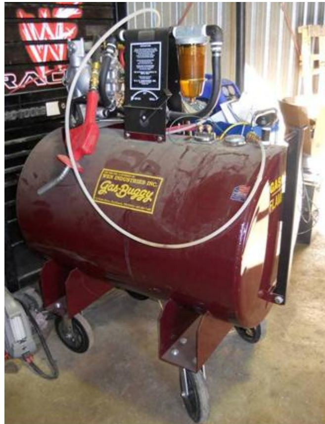
Figure 2: Example of Gasoline Collection System
