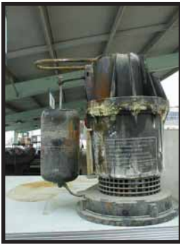
A mercury-free sump pump. Notice the metal guide and no attached wires.
