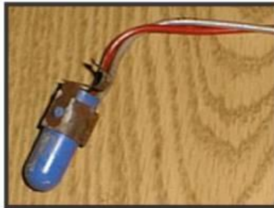
Figure 7: Washing Machine Mercury Switch (Source: Vermont Department of Environmental Conservation et al., 2002)
