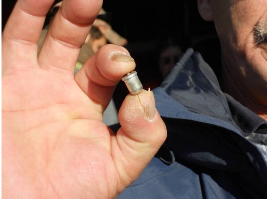
Figure 11: Mercury Pellet from Vehicle Convenience Light Stockpiling
