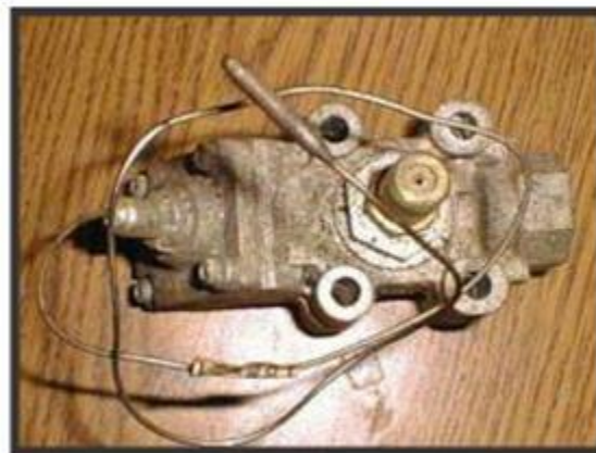
Figure 8: Gas Safety Valve Control, Gas Safety Valve Capillary Tube and Safety Valve Sensor Bulb from Gas Range (Source: Vermont Department of Environmental Conservation et al., 2002)
